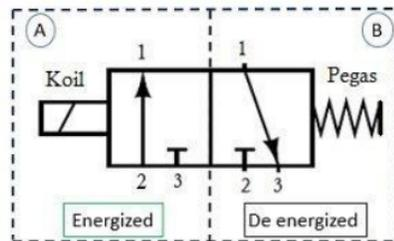
■ Gambar 2. Diagram 3 Way Solenoid Valve
