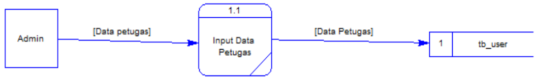
Gambar 4.5 Data Flow Diagram Level 2 Proses 1
