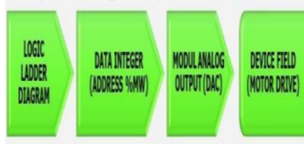
Gambar 4.4 Alur proses sinyal analog output
