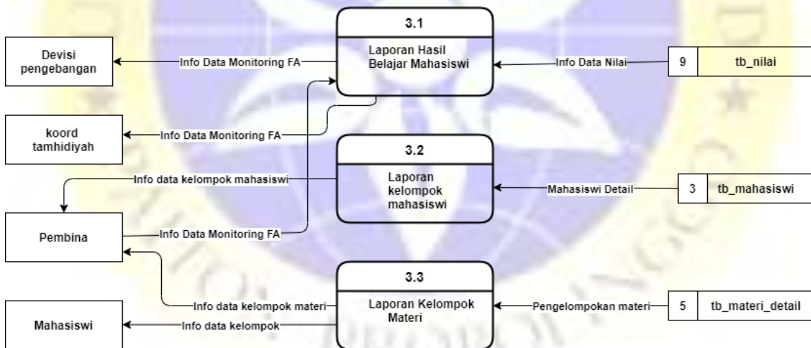
Gambar 4. 9 DFD Level 2 Proses 3 Laporan Monitoring
