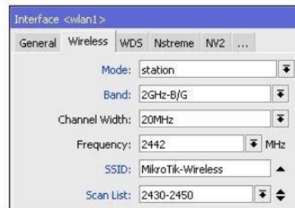
Gambar 19. setting wireless station (client).
